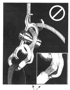
Make sure your carabiner is properly aligned and oriented before loading the SCARAB®, particularly on rappel. Small carabiners can sometimes jamb inside a Hyperhorn. This could possibly damage the carabiner or even lever the gate open. Pay attention to your system, before you weight it!
