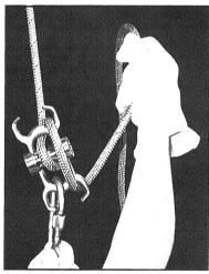
2) To add friction, wrap the in feed line around a rear horn (anchor or harness side) on the same side as you began with.
