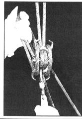
With small diameter ropes (not certified for NFPA G), such as this 8.1mm half rope, it is possible to rig two strands as if they were one strand of rope. Many configurations are possible depending on the diameter and construction of rope used.
