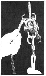
3) For rescue sized masses (200kg) cross to the empty forward Hyper-horn. For even more friction (for 280kg) wrap the remaining horn.
